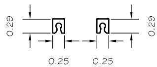
13 - FULL BREAKOUT TRACK 6063-T5 ALLOY
